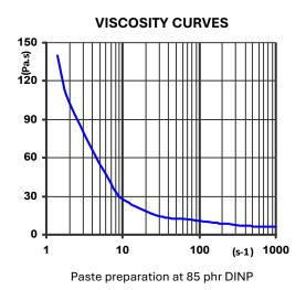
**Characteristics** Units Values **Standards** Viscosity index ml/g 124 ISO 1628-2 K value (cyclohexanone) 70 ISO 1628-2 Polymerization degree 1200 Particle size on 120 mesh (0.125 mm) ≤ 0.015 ISO 787-18 % ISO 1269 Volatile matter % ≤ 0.3 Residual Vinylchloride monomer **ASTM D3749** ≤ 1 ppm
